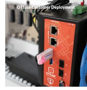
Once switched into 'Protection' mode, the OTfuse will apply its customized policy to the Endpoint Segment assets directly and in real time, while alerting the customer via their existing SCADA system of any blocked events. Customers can interact with a single OTfuse directly from their control room, or make use of a centralized web-based management console for batch review of policies and events across a large number of individual appliances.
